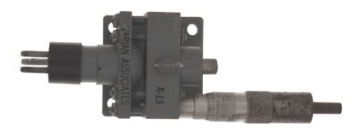
Innovator image: X-13 Klystron tube, n6jv.com collector`s website
